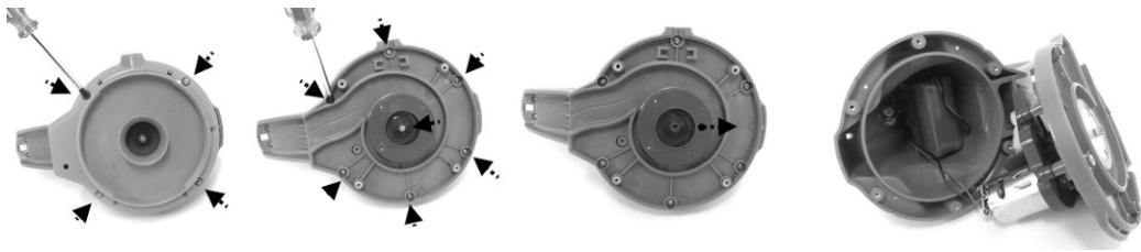
3. Remove out the battery pack to expose the PCBA. To detach the battery connection wire, press on the clip of the connector to pull it out. NOTE: Wrap the connector immediately with insulating tape in order to avoid any short circuit caused by the contact of both wire terminals.
