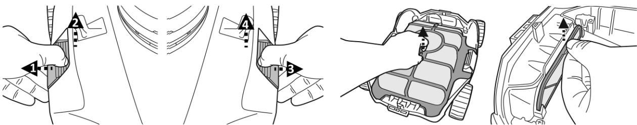
2. Detach the filter cover and filter plate and remove the debris from the compartment. It is recommended to clean the filter cover net and draining filter plate with splashing water. If brushing is deemed necessary, use only a soft brush to clean it carefully and gently to avoid damages.
