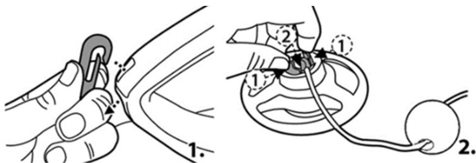
Release the retrieval cord from the stem to a length equivalent to the distance between the handle of the robot and the water level. **NOTE:** Excess length may kink the rope and affect performance as a result.
