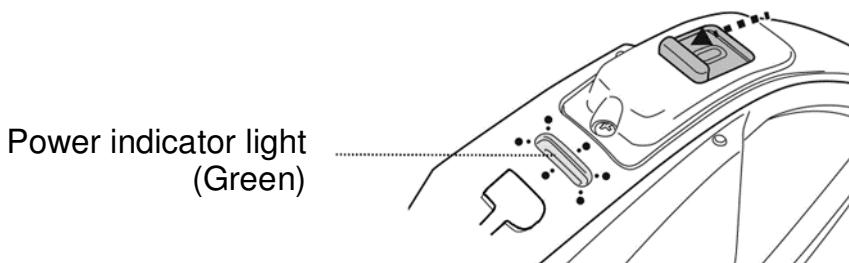
3. Slide the power switch to “ON” (while the robot is still submerged) – the indicator light will turn on and activate the motor automatically (water level covering the sensors at the top of the swivel head). Let the robot sink to the pool floor and observe its first forward and reversed movements across the pool bottom. If it runs along the pool wall instead of
