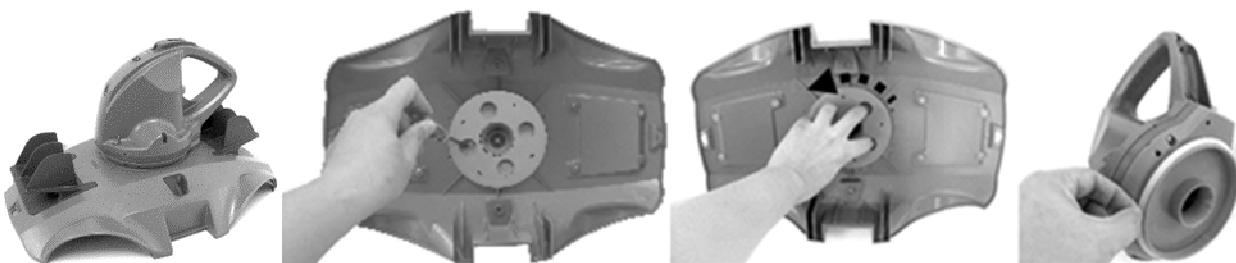
2. Use the screwdriver to unscrew the 4 screws located at the bottom of the head to release the bottom plate first. Then unscrew all the screws at the base as shown. Remove the impeller and pry open the base to expose head inside.
