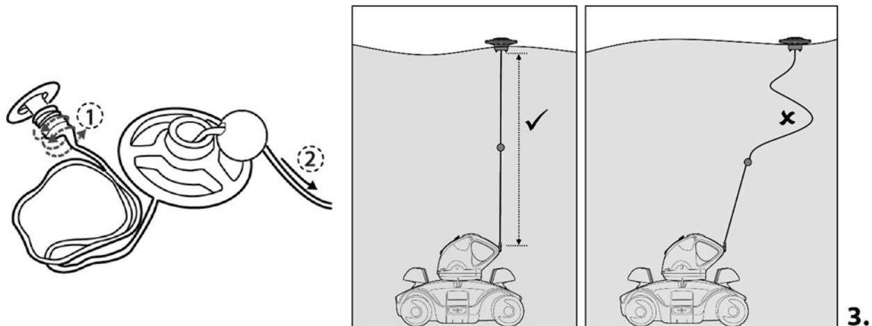
Once the desired length has been achieved, maintain it by holding the rope onto the stem and reattach it to the float by pressing on the side clip as shown.
