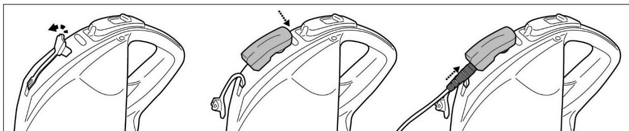
3. Connect the external adaptor to the power source. The indicator light on the external adaptor turns red once the charging begins. The indicator light on the external adaptor will turn green when the robot is charged.
