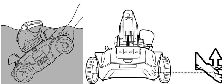
5. Slide the power switch OFF. Rinse the robot with fresh water after every use. DO NOT use any detergent.
